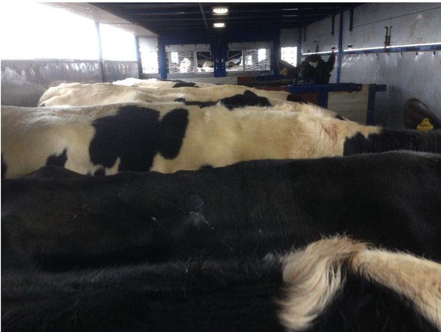
Figure 4. A typical view inside a truck loaded with cull cows. They all stand perpendicular to the direction of driving and are not tied. Partitions divide the space into smaller units to prevent the cows from moving too much around and reduce the risk of falling.
