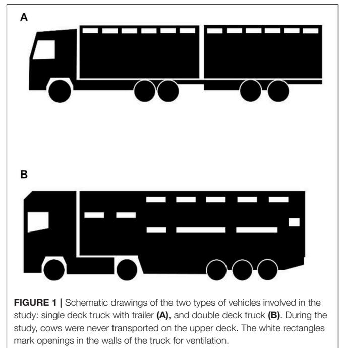
**FIGURE 1** | Schematic drawings of the two types of vehicles involved in the study: single deck truck with trailer (A), and double deck truck (B). During the study, cows were never transported on the upper deck. The white rectangles mark openings in the walls of the truck for ventilation.
